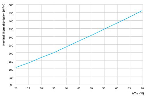
The specified nominal thermal emission applies at a turbulent flow rate of 0.015 l/s. If the flow rate is lower, the output will decrease and the calculated output will be reduced according to the output factor diagram below.
